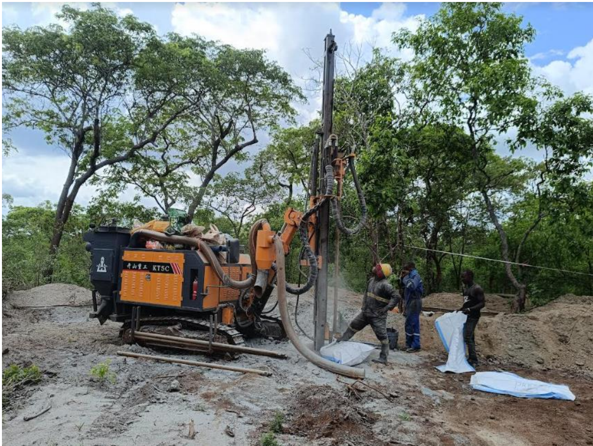
RC Drilling at site
